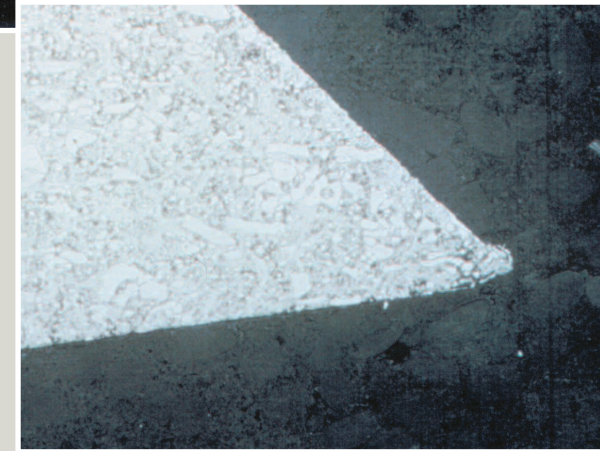
The tip of a hand-honed slitter blade is shown in the top photo (.001 radius at the tip). The lower photo shows the tip of a superfinished slitter blade after sharpening by Valley Grinding (.0001 radius at the tip). Both photos are at 400x magnification.
